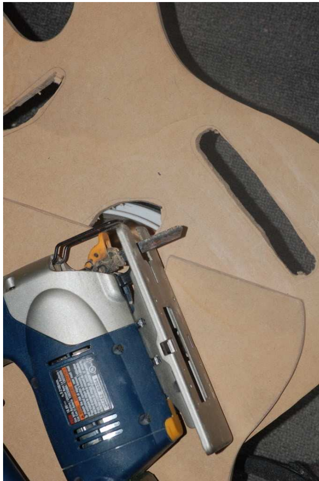
Fig. 10 cut close to the pencil line but not to close
