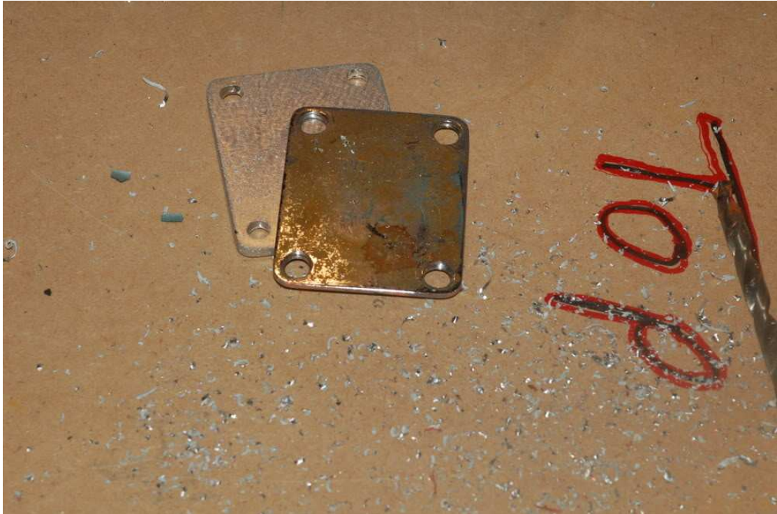
Fig. 13 neck plate made from a piece of aluminum scrap
